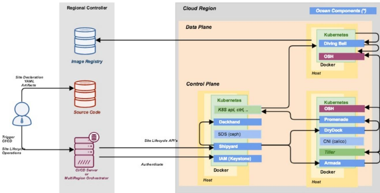
AT&T is finding that containerization allows them to shift traditional deployment-type activities far to the left, and to validate them using CI/CD. Kubernetes additionally provides massive scalability and resiliency, as well as hooks to allow OpenStack-Helm to declaratively configure operational behavior, inject configuration, and accomplish rolling upgrades and updates without impacting tenant workloads.
