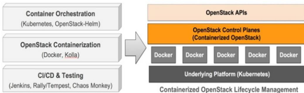
SKT specifically emphasizes an automated continuous integration/continuous delivery (CI/CD) pipeline around containerized Openstack on Kubernetes. SKT's CI system consists of [Jenkins](#), [Rally](#), [Tempest](#), Docker Registry, as well as Jira and Bitbucket. SKT also developed an open source tool called [Cookiemonster](#), a chaos-monkey like resiliency test tool for Kubernetes deployment that performs resiliency tests for their CI pipeline.
