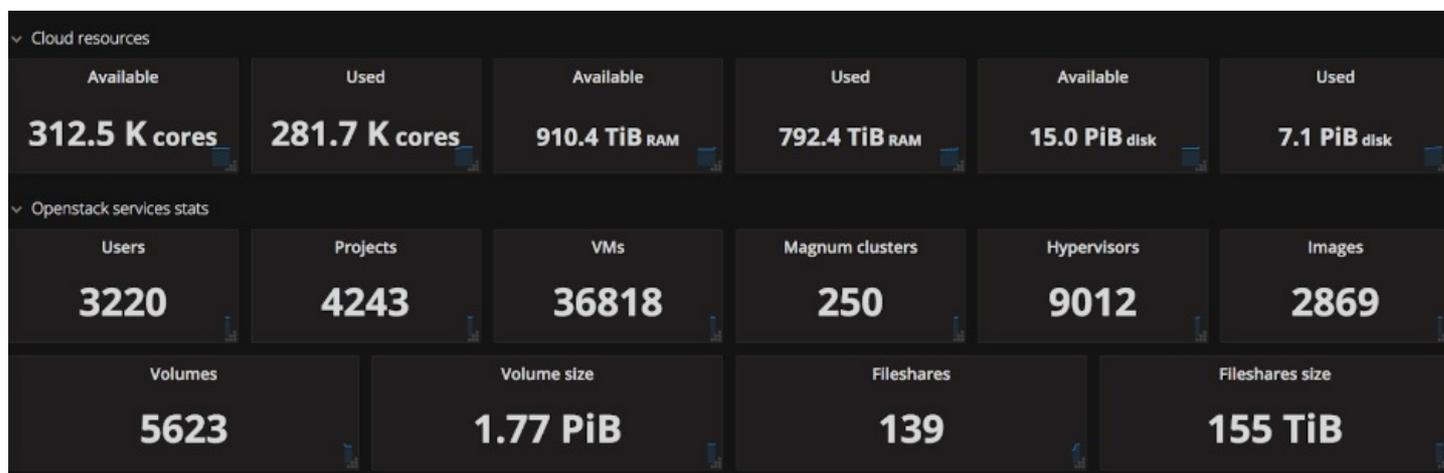
CERN's OpenStack cloud gives users self-service access to request a configured container engine with a couple of commands or via a web GUI. This allows rapid utilization of the technologies and can scale to 1000s of nodes if needed. Best practice configurations are available with built in monitoring and integration into CERN storage and authentication services.
