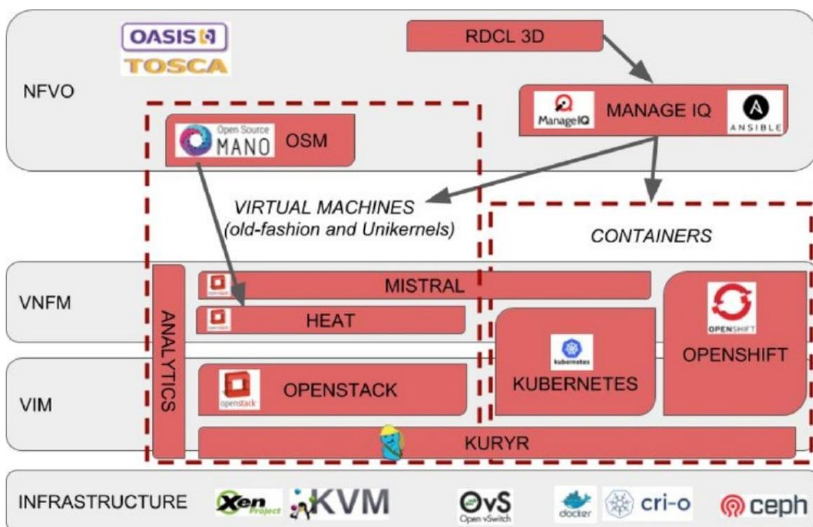
By leveraging Ansible playbooks executed from the ManageIQ appliance, SUPERFLUIDITY offers a common way to deploy applications. These applications in turn use the cloud orchestration functionality provided by OpenStack Heat templates and OpenShift templates.
