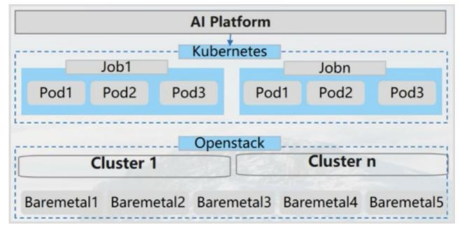
*Training scenario:* Baremetal is scheduled to implement model training. *Inference scenario:* The application runs on the virtual machine, and the model runs on the baremetal.
