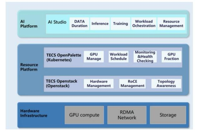
Architecture: ZTE has launched a three-tier software architecture to solve the problem of Al:
