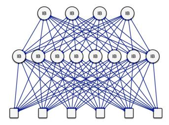
An example InfiniBand network fabric, in a fat tree topology, in which each compute node (bottom row) has 8 InfiniBand links. Multiple links may exist between switches to produce a non-blocking network, in which all nodes could communicate simultaneously on all links at full network bandwidth.
